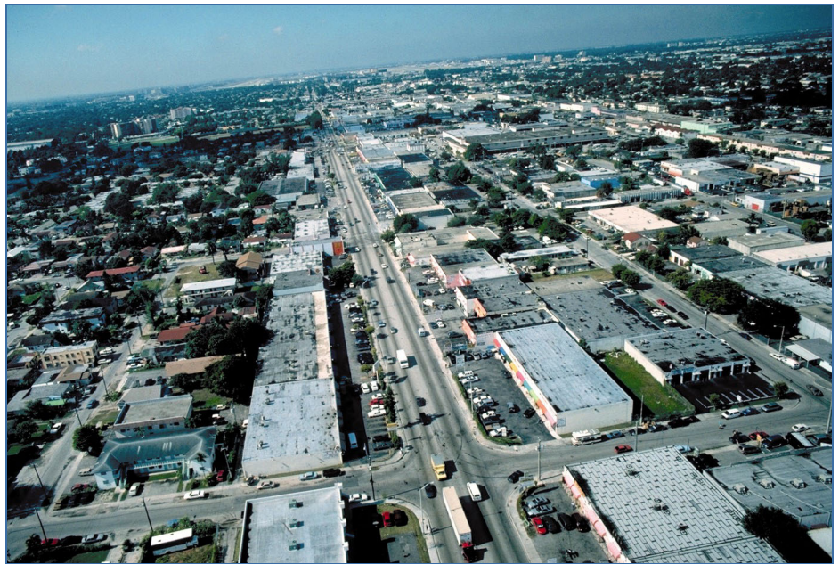
Figure 3. Urban areas contain a great deal of impervious surface that accumulates pollutants and transports runoff rapidly to receiving waters
