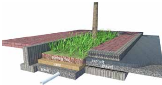
Above: Cross-section of stormwater planter. Right: Stormwater planters along Rockville Pike in Rockville, MD.
