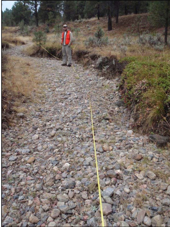
Figure 22. Stream channel with headcuts and grade controls “absent” (Blue Mountains, channel width 2.4 m)
