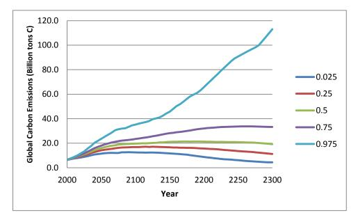
Figure 5-5: Extrapolation of Global CO2 Emissions to 2300, Assuming Rate of Change of Carbon Intensity declines linearly to zero by 2300.
