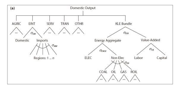
Figure 3-1: Example of the nest structure for production sectors in EPPA: parameters that govern energy demand (and abatement costs) are substitution elasticities for energy—non-energy,  $\sigma_{EVA}$ ; labor-capital,  $\sigma_{VA}$ ; electricity-fuels,  $\sigma_{ENOE}$ ; and that among fuels,  $\sigma_{EN}$ .
