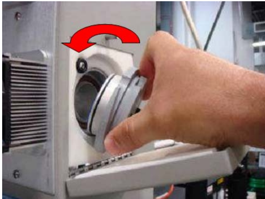
Figure 10-21. Photograph illustrating removal of the 47-mm cartridge and filter.
