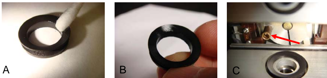
Figure 10-11. Photographs illustrating application of silicone grease to the V-seals and O-rings (Panels A, B) and repositioning of the brass bushing on the motor cam post (Panel C, arrow).
