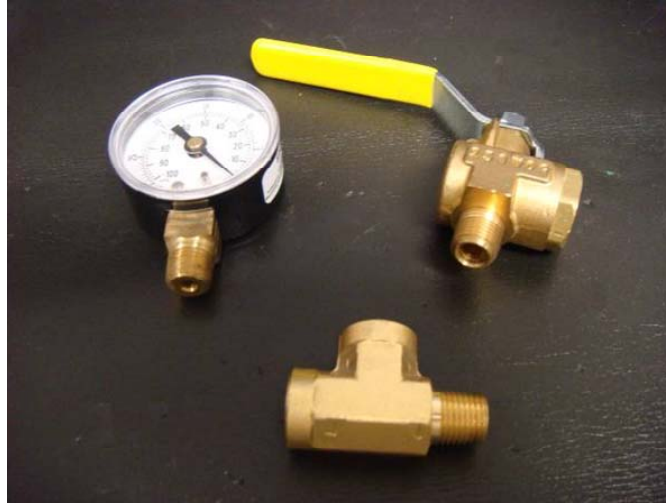
Figure 10-1. Photograph of the additional plumbing parts needed to conduct the full system leak check.
