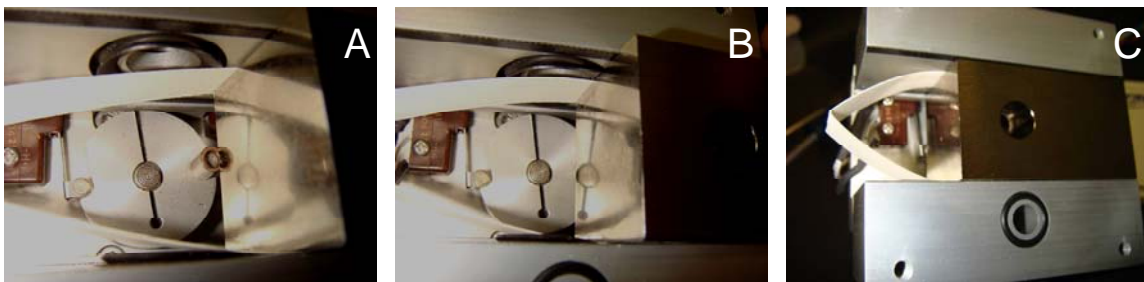
Figure 10-13. Photographs illustrating installation of the diverter block by working the folded paper under the top and bottom edges of the block (Panel A) so the paper prevents the seals from rolling as the block is reinserted (Panel B) and the block is properly aligned with the bushing on the cam pin. The block can then be pushed back so its front face is flush with the upper and lower housing plates (Panel C).
