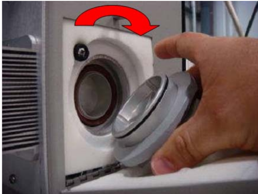
Figure 10-23. Illustration of the chiller cap replacement. For chiller cleaning, replace the chiller cap without the 47-mm filter holder.
