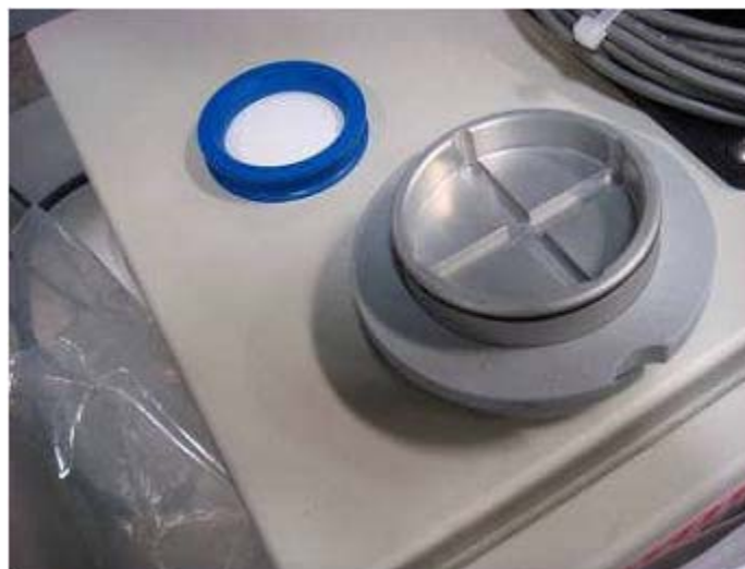
Figure 10-22. Example of a clean chiller cap. The chiller cap should be wiped clean of any residue at the beginning of the chiller cleaning process.
