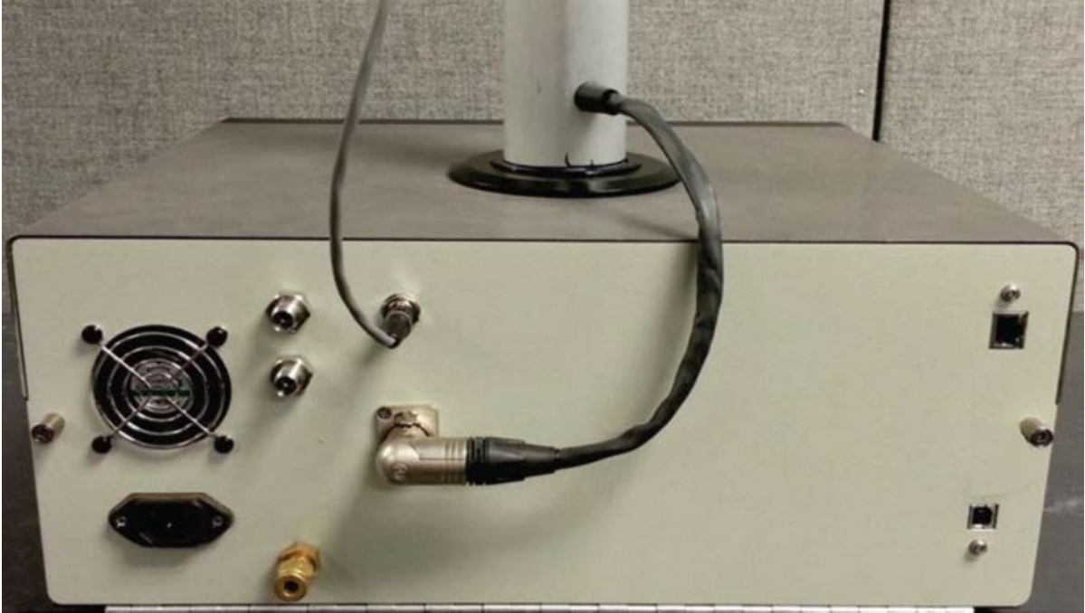
Figure 25. Ambient Temperature Probe and ASC Connections
