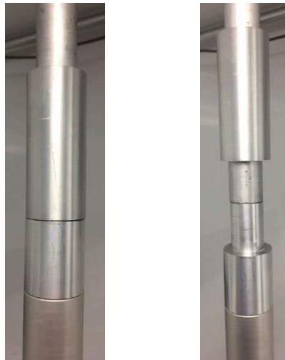
Figure 12. Slip coupler in normal position and lifted vertically.
