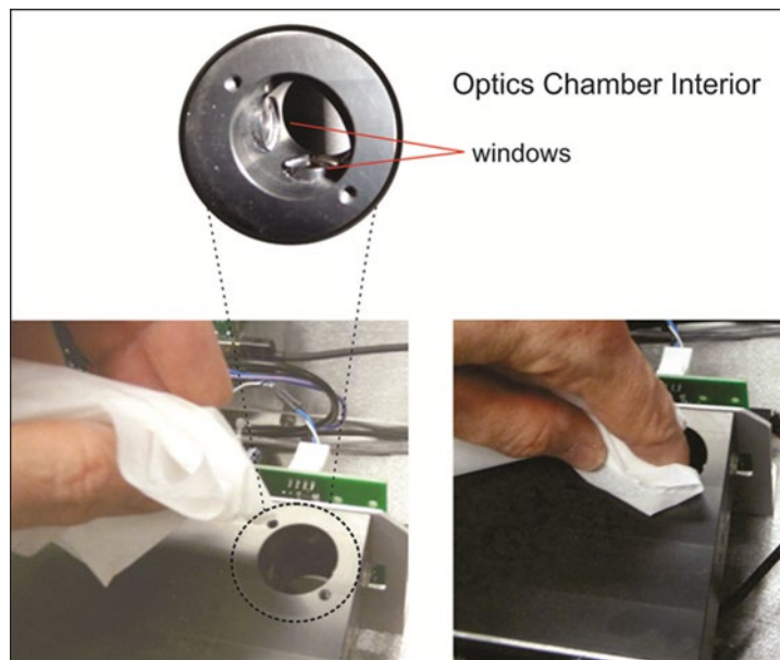
Figure 10. Maintenance: Optics Chamber Windows
