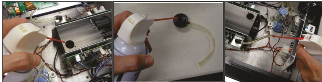
Figure 11. Maintenance: Final Dusting
