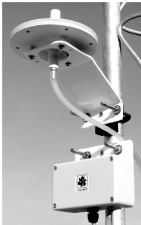
Figure 7.4 Tower-Mounted Barometer with Pressure Port. Source: http://www.youngusa.com
