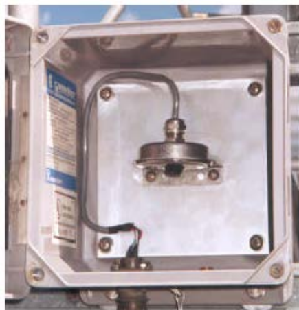
Figure 7.3 NEMA 4X Enclosure. Source: http://www.climatronics.com/pdf/products/sensors/102270.pdf
