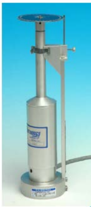
Figure 2.17 Linearity Test Fixture
