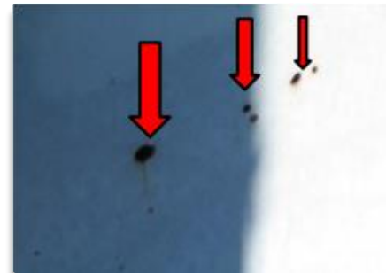
Holes in Tanks
