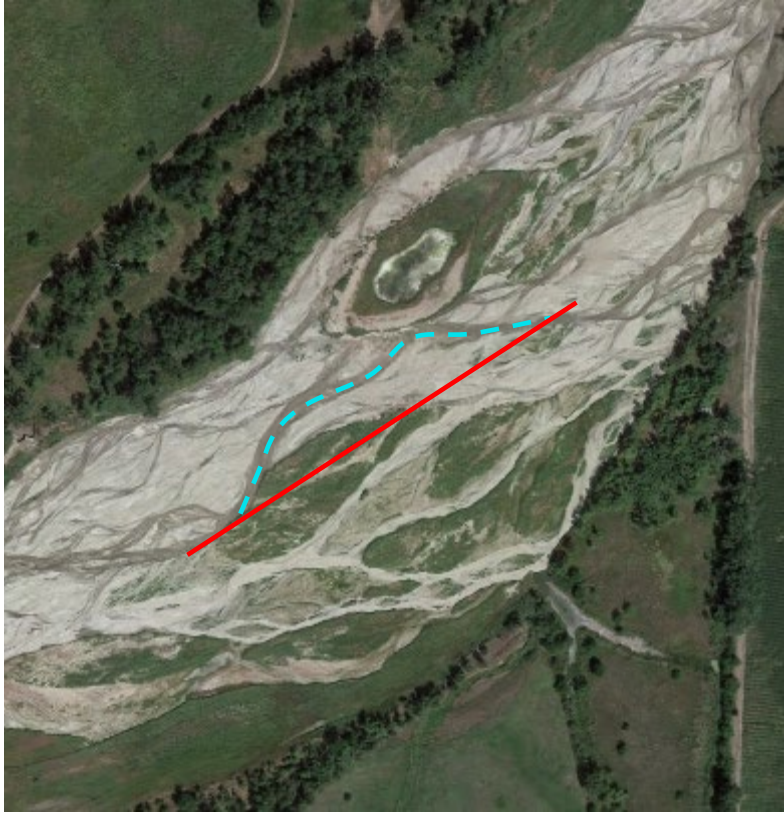
Figure 17. Sinuosity measurements in a multi-threaded system. The stream length (dashed blue line) is measured in the dominant (i.e., lowest elevation) channel. Valley length is represented by the solid red line.
