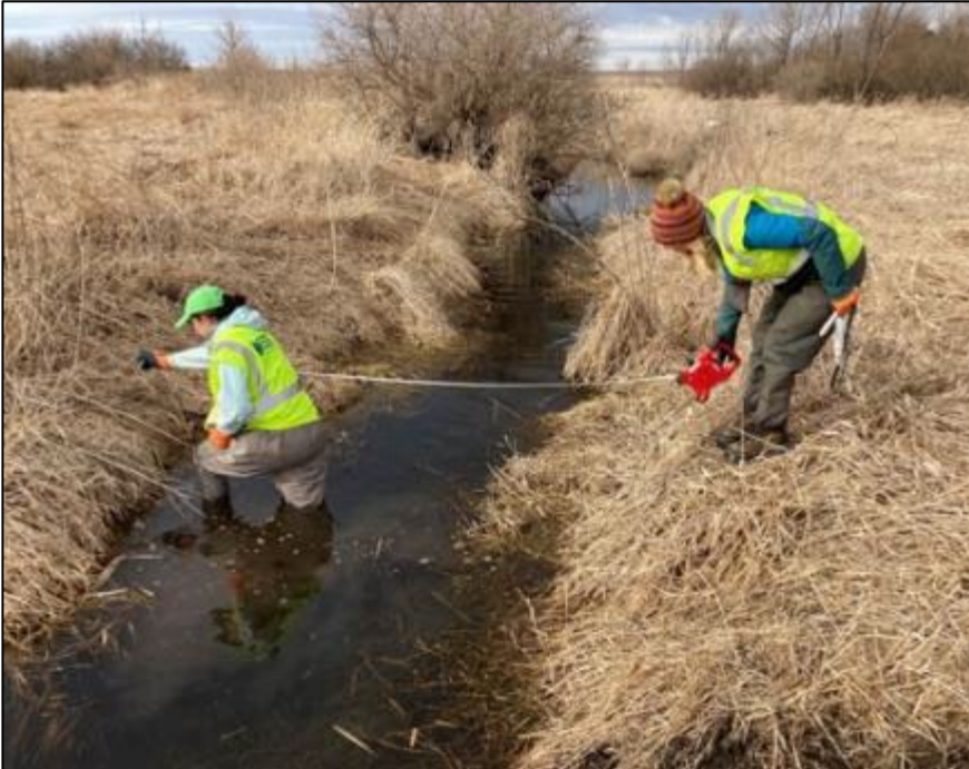
Figure 5. Measuring bankfull width. Image credit: James Treacy
