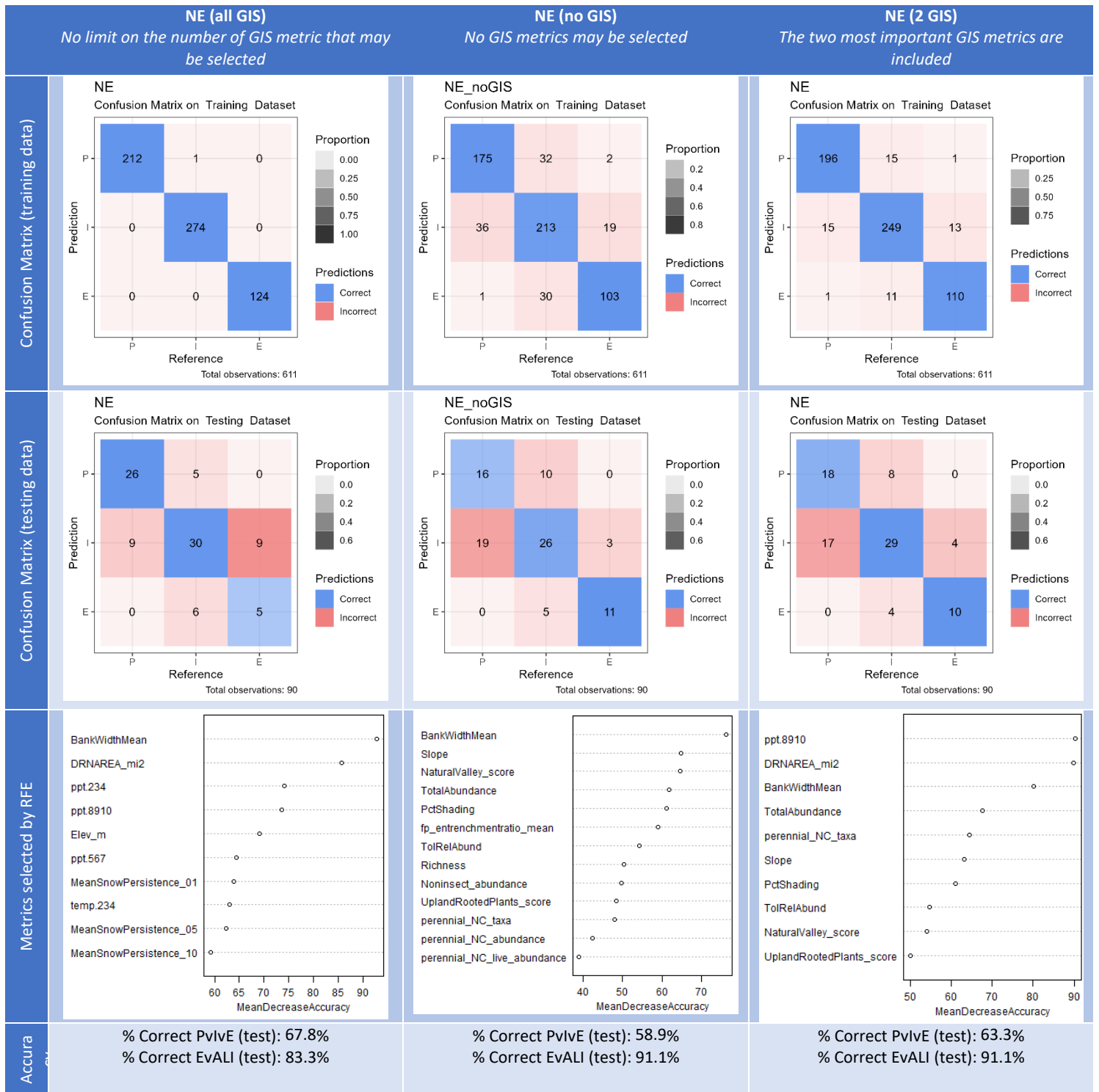
Figure 16. Detailed performance of the three Northeast Models (all GIS), (no GIS), and (2 GIS) (see Table 6 for descriptions). The top row provides confusion matrices for the training data and the second row shows confusion matrices for the testing data. Shading of boxes in matrices describe the proportion of samples in each dataset. The third row lists the metrics selected by Recursive Feature Elimination for each model (with metrics at the top having greater importance in terms of contribution to model accuracy). The bottom row lists the accuracy metrics PvlvE and EvALI on the test data.
