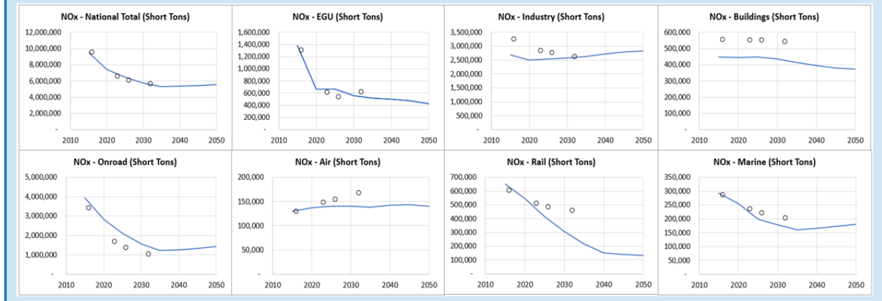
Figure A-2.45: Comparison of GLIMPSE-1.1-Ref NO x emission projections, in total and by sector (lines), with those of the EPA 2016v2 emission platform (dots).
