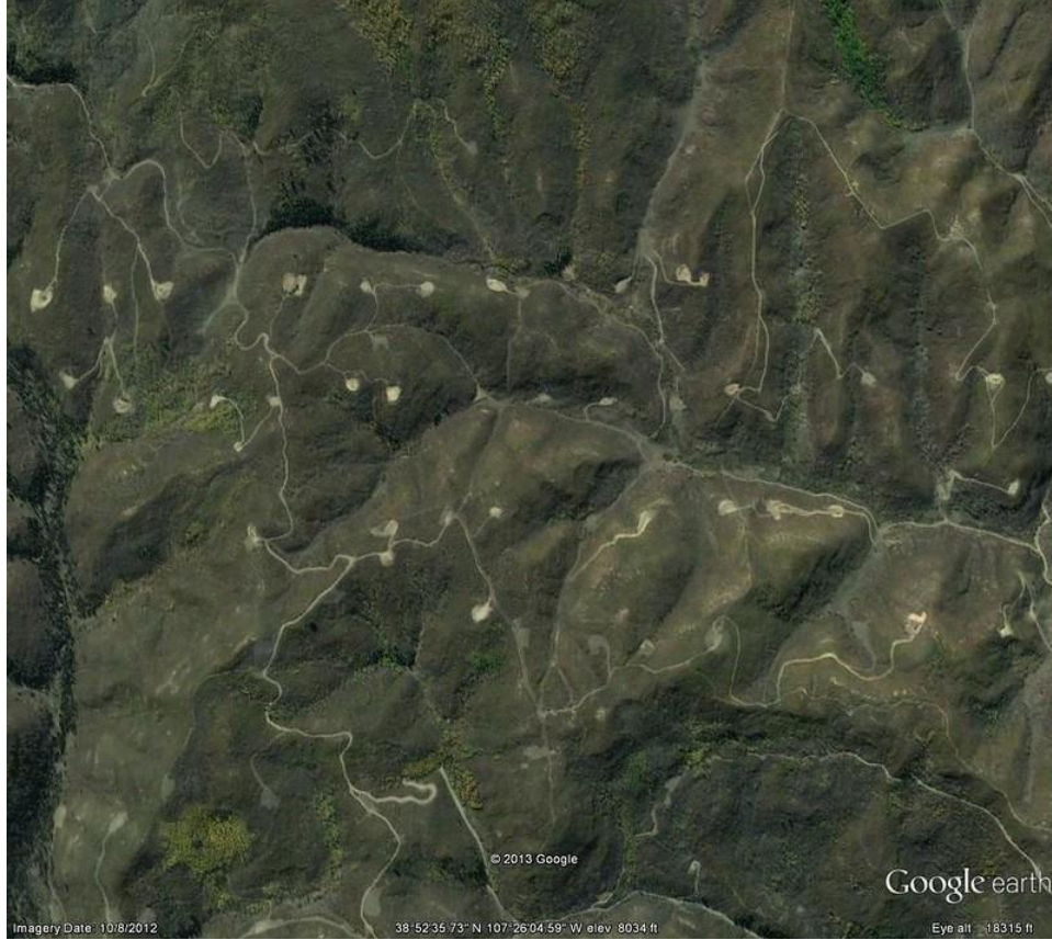
Figure 6: Satellite view of the extensive system of mine ventilation boreholes developed above the Mine
