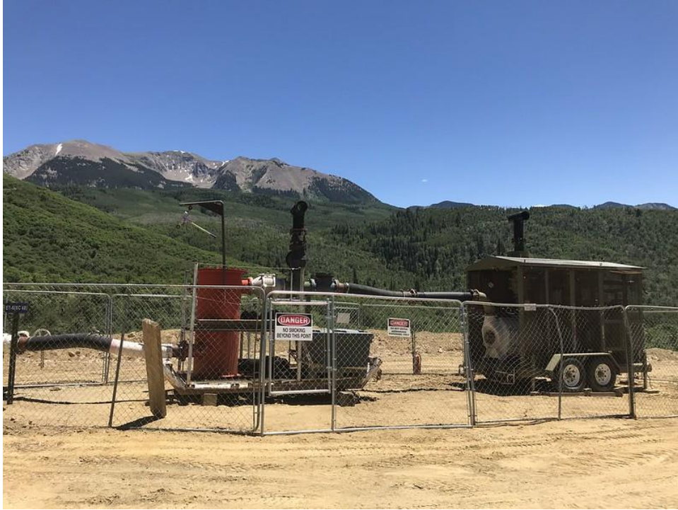
Figure 4: Mine ventilation borehole operating above the West Elk Mine
