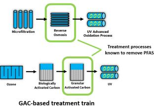
RO-based and GAC-based advanced treatment trains used to purify treated wastewater prior to conventional drinking water treatment. These are two example treatment trains; there are other possible
