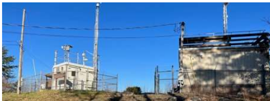
Figure 3 Look Rock CASTNET site located in Great Smoky National Park (GRS420, TN) is co-located with IMPROVE (Integrated Monitoring of Protected Visual Environments) and the Atmospheric Science and Chemistry Measurement Network (ASCENT). IMPROVE provides speciated measurements of PM constituents. ASCENT will provide high-time resolution measurements of black/brown carbon, PM speciation, metals and PM size fractions at three CASTNET sites.
