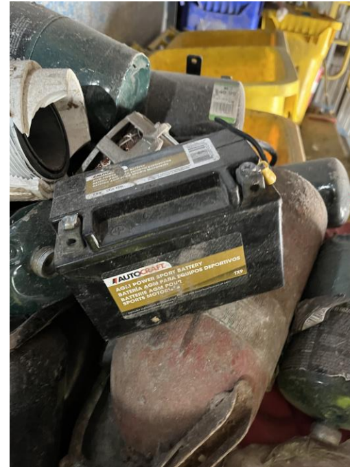
Photo 2: A mid-format battery was collected and sorted out of a recycling facility
