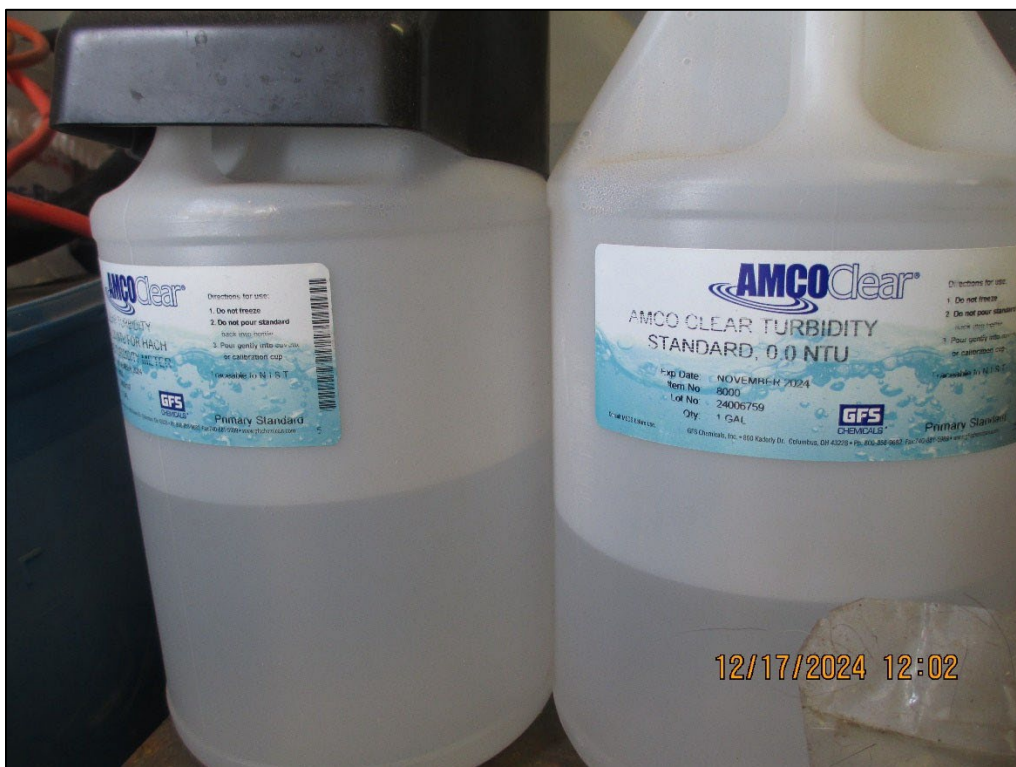
Photograph 16. The turbidity standard reagents were expired in November 2024.
