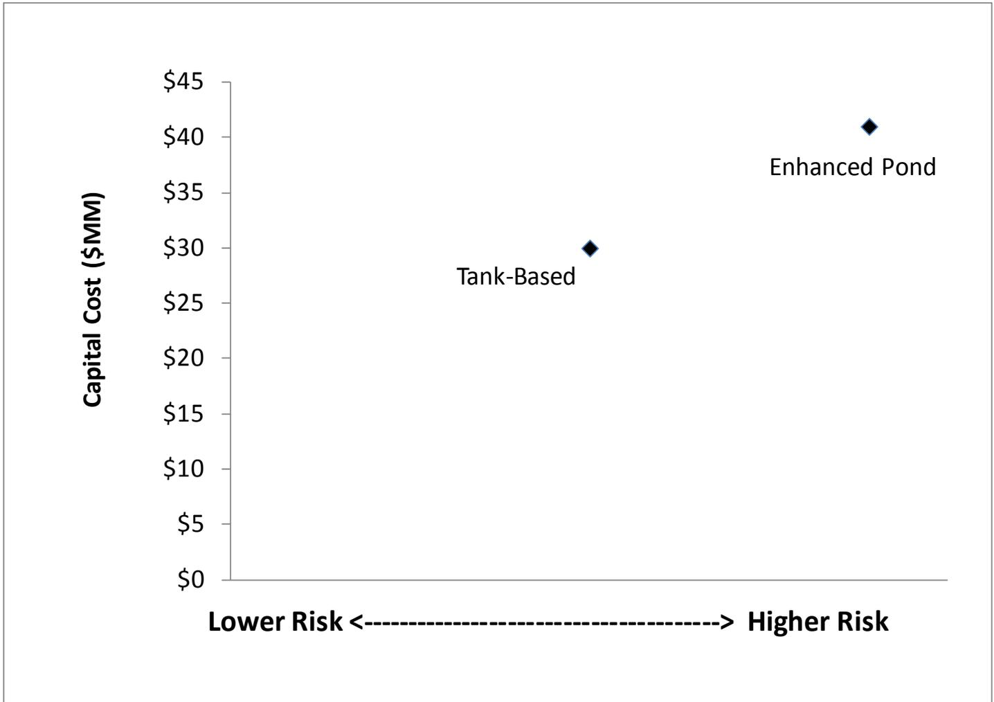
Due to land restrictions at the facility, there is no room to build the enhanced pond other than on top of retired ash pond unit(s). Risks associated with enhanced pond treatment include:
