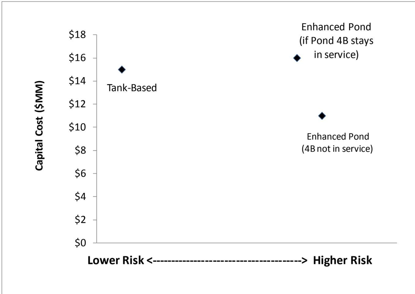
Due to land restrictions at the facility, there is no room to build the enhanced pond other than on top of retired ash pond unit(s). The cost of preparing Pond 4 for construction of an enhanced pond is higher if Pond 4B needs to
