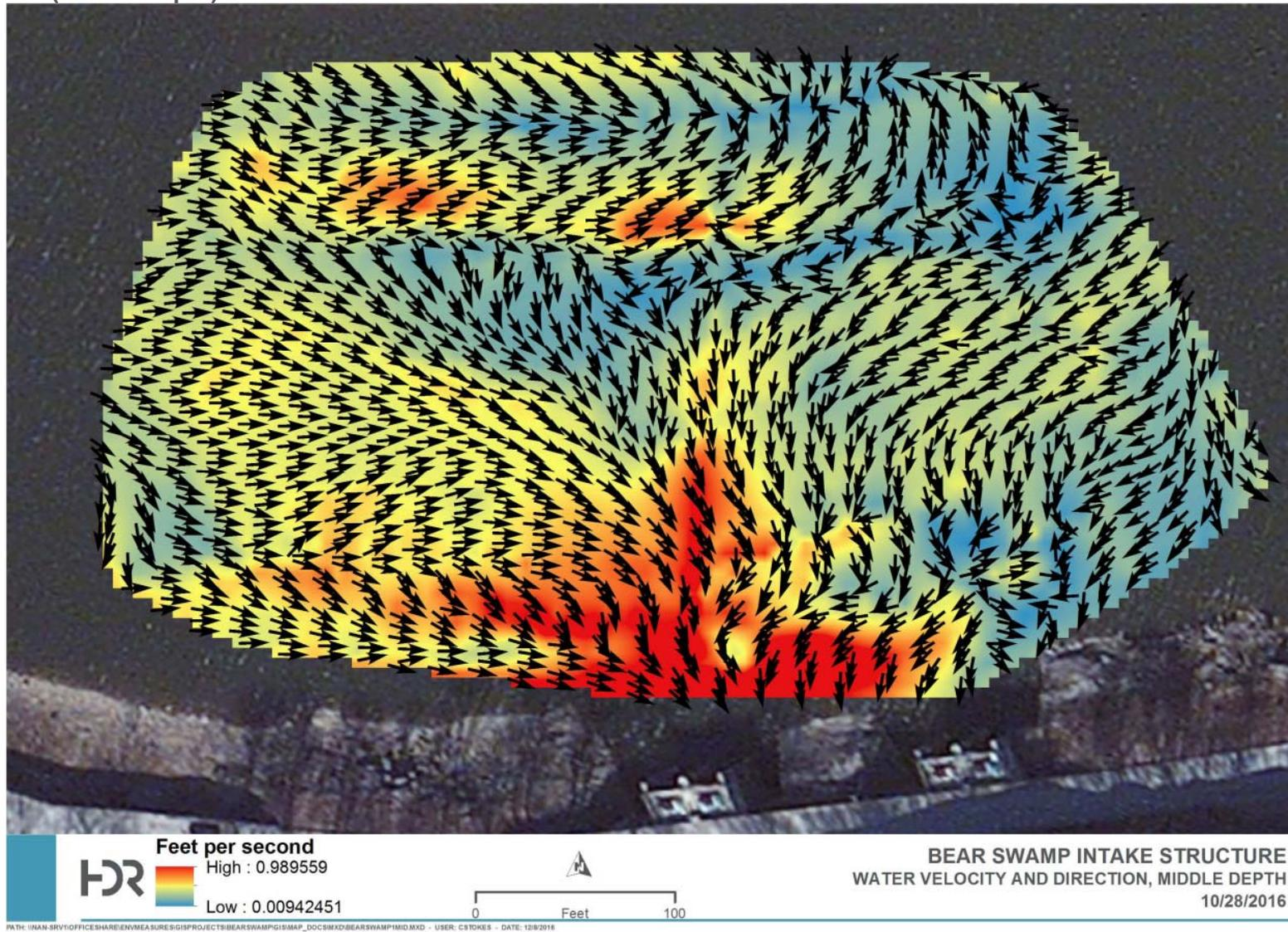
Figure 5-5. Bear Swamp PSD Unit 2 Pump Operation at Nominal Lower Reservoir Elevation of 836 feet, Water Velocity and Direction (Surface Depth)
