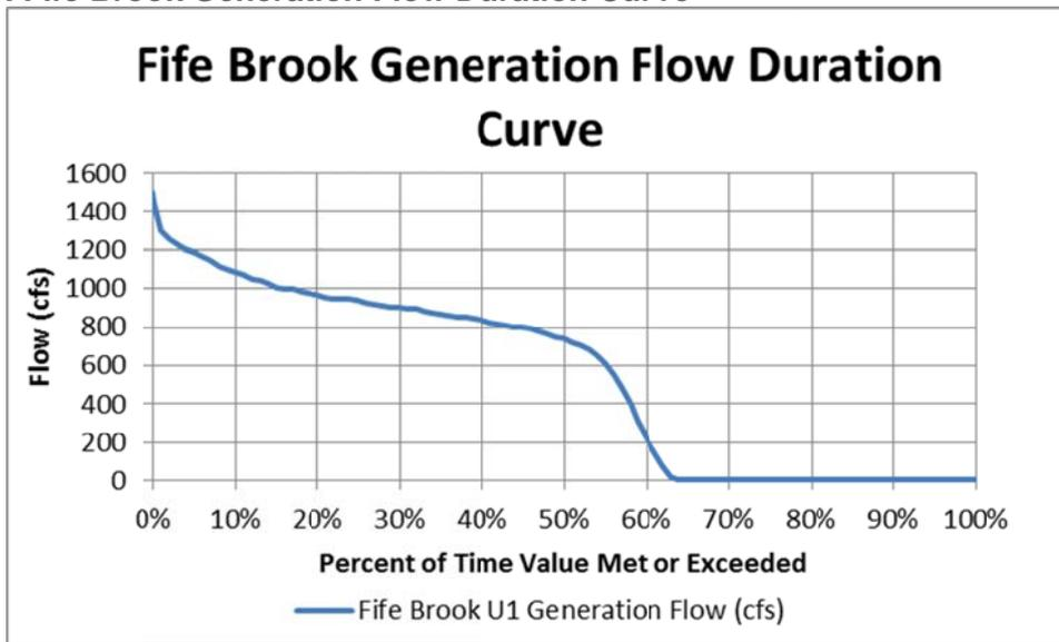
With this, the total flow area at the face of the trashracks (552 square-feet) can be applied to the flow ordinates within the generation flow duration curve to derive a Fife Brook generation velocity duration curve as shown in Figure 5-10 below.
