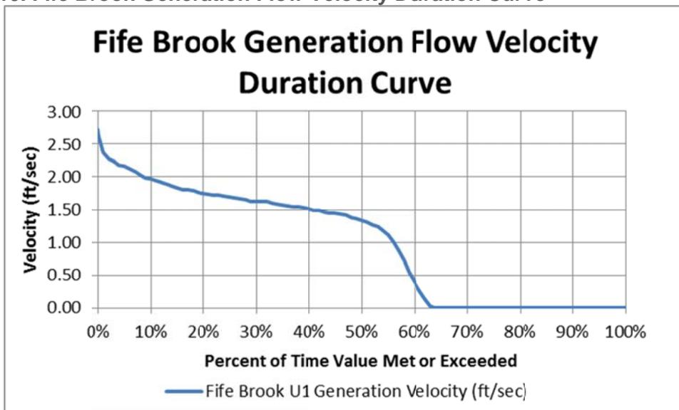
As depicted, maximum velocities at the face of the deeply submerged trashracks are calculated to be approximately 2.7 fps with velocities at or below 2 fps 92 percent of the time.
