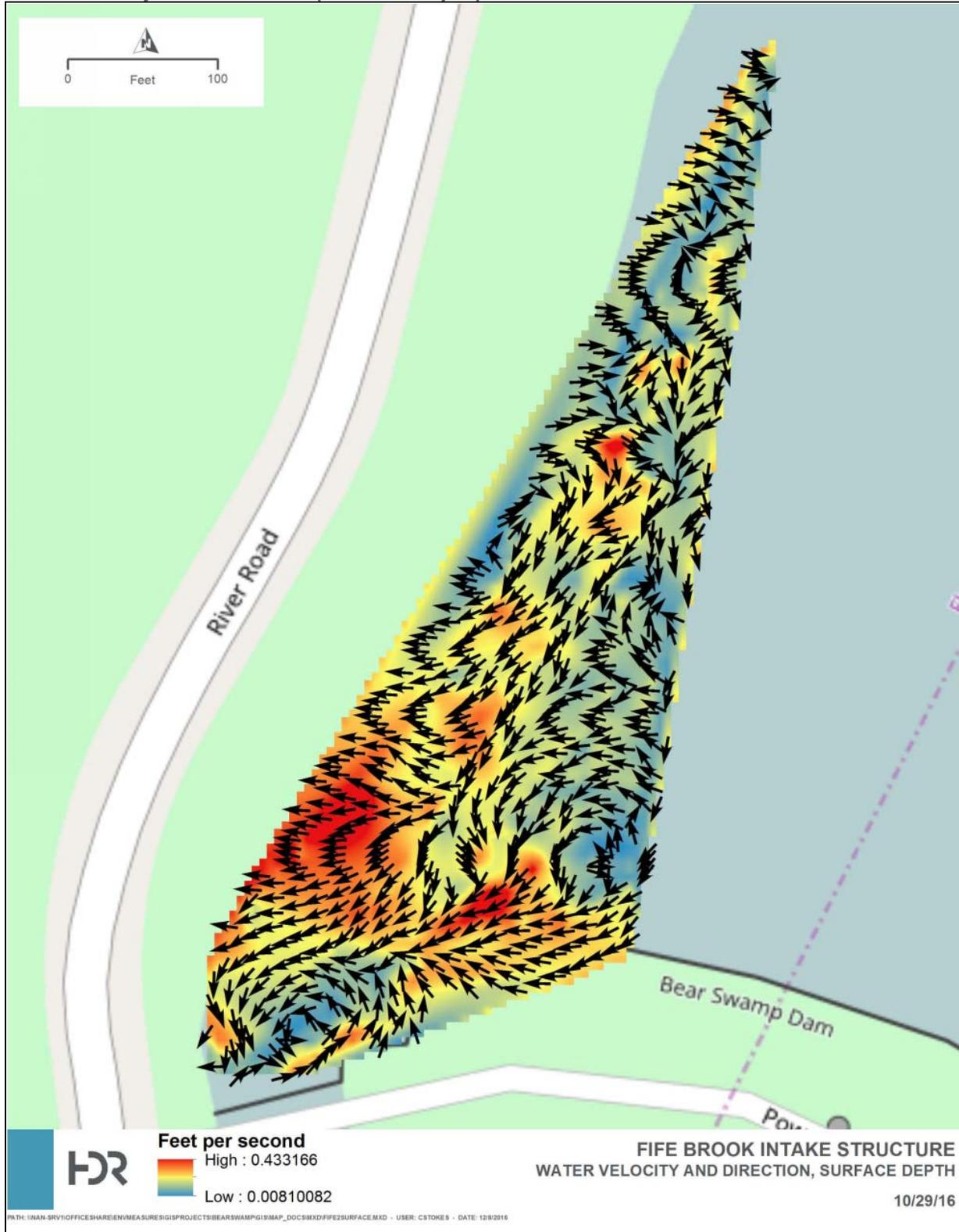
Inasmuch as velocities one foot upstream from the face of the trashrack are calculated as approximately 0.68 fps based on historical data (and could reach 0.7 fps if the maximum generation flow rating of 1,540 cfs were achieved); key observations include:
