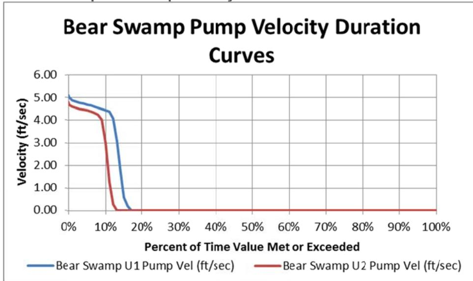
As depicted, the maximum velocities immediately at the face of the Unit 1 and 2 trashracks (approximately 5.1 fps and 4.8 fps respectively) are short-lived with the velocities being between 4 and 4.5 fps during the majority of the pump cycle.
