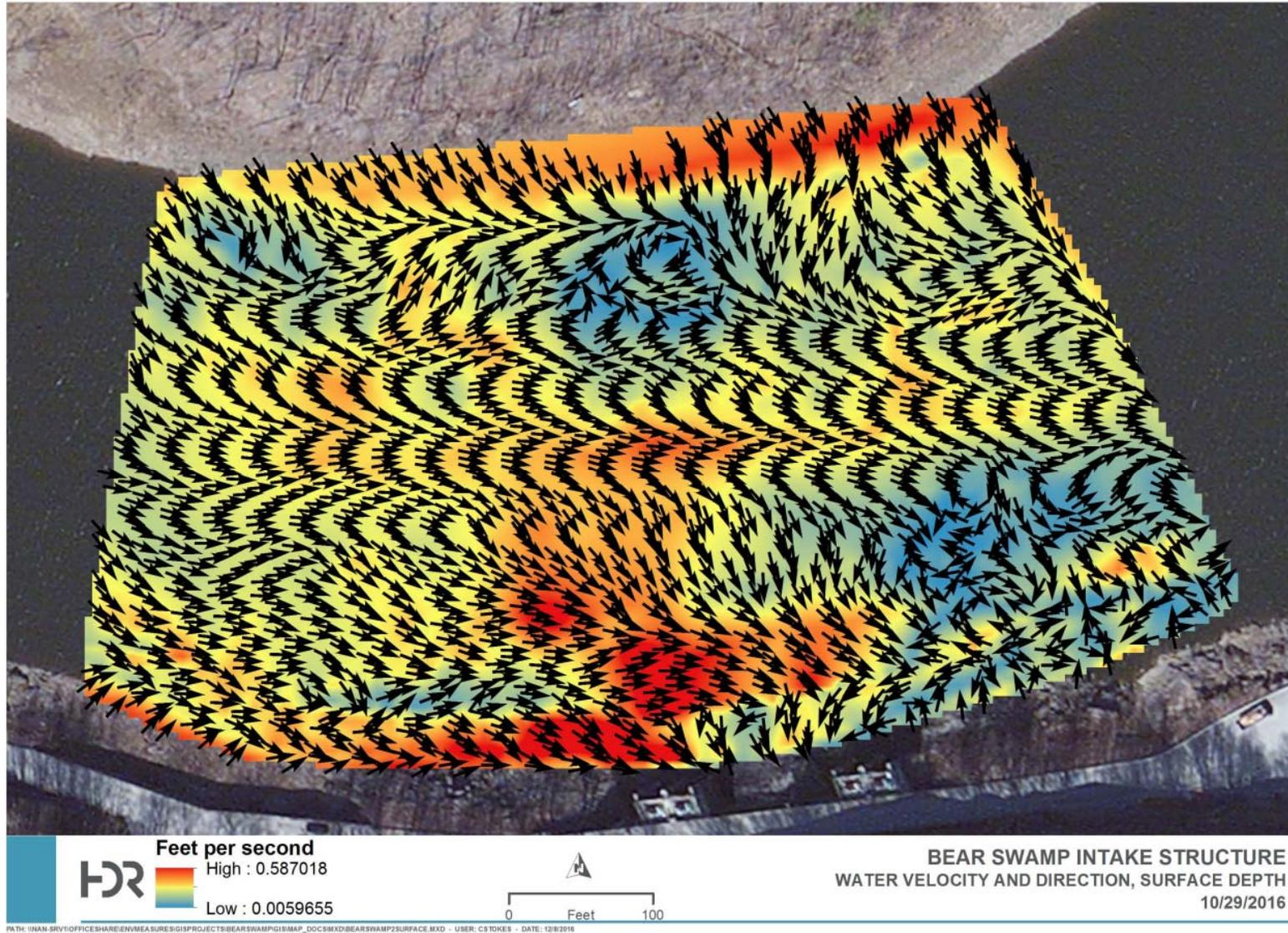
Inasmuch as velocities at the face of the Unit 1 and 2 trashracks are calculated as approximately 5.1 fps and 4.8 fps, respectively, based on historical data (and could reach 5.4 fps if the maximum pump flow rating of 4,520 cfs were achieved); key observations include:
