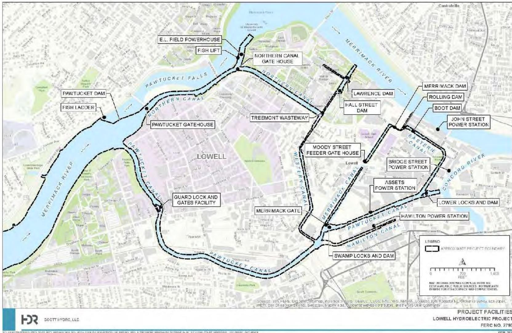
Figure 2–1. Major features of the Lowell Hydroelectric Project.
