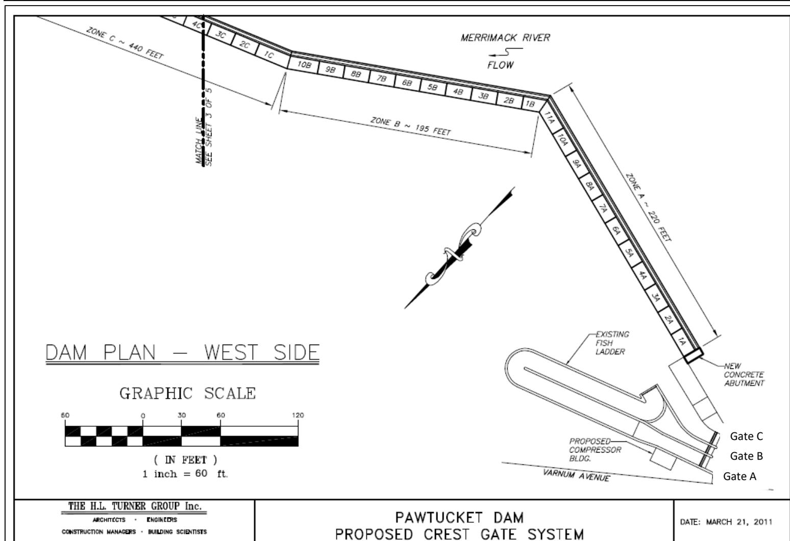
Figure 2-2. Pawtucket Dam fish ladder, through-water supply (gate A), supplemental attraction water gates (gates B and C), and zones A-C of crest gate system.
