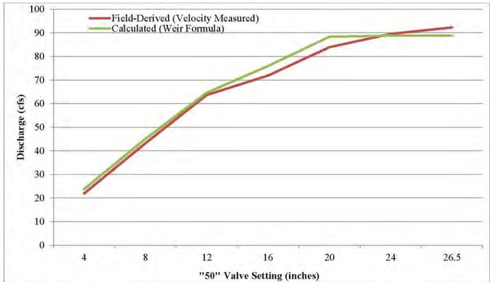
Figure 1. Rating curve showing "50" supply settings and resulting discharge over the entrance weir crest at the Lowell Hydroelectric Project.
