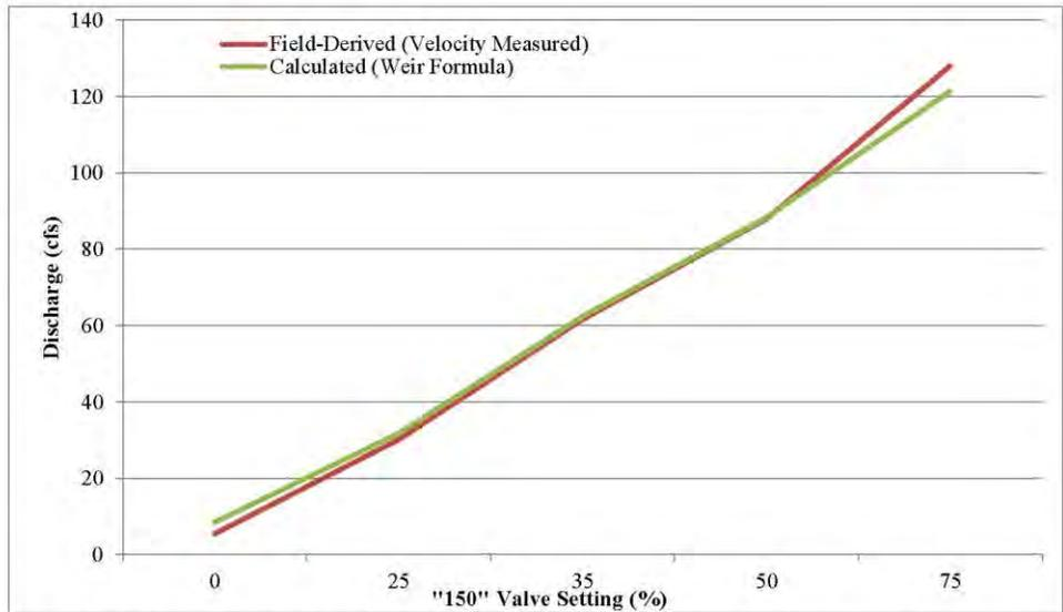
Figure 2. Rating curve showing "150" valve settings and resulting discharge over the entrance weir crest at the Lowell Hydroelectric Project.
