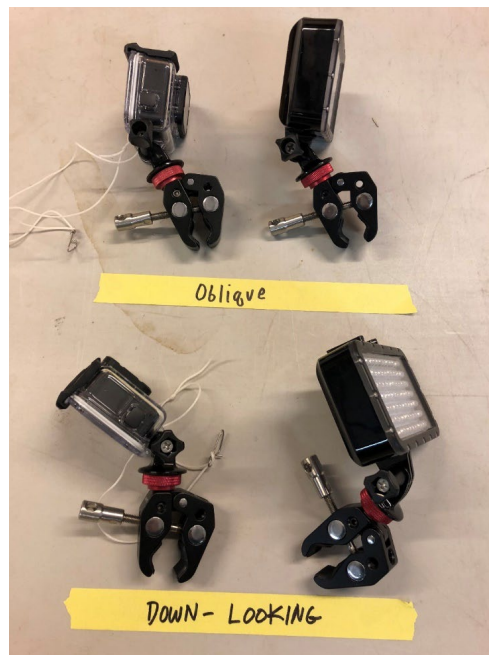
Appendix D Figure 3. Approximate aiming angle of camera and lights for the oblique (B) and down-looking (A) cameras. Note the orientation of the tripod adapter (the fitting between the red locking thumbscrew and the camera or light) which is facing backward relative to the camera lens.
