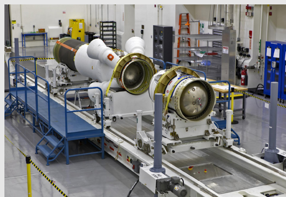
One of the Launch System Abort motors for NASA's Orion spacecraft was built and tested at the Elkton plant.
