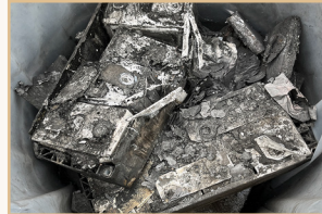
Crews contain batteries in lined drums for safe transport to staging areas.
