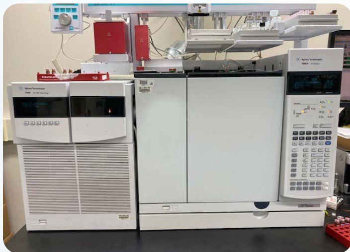
Figure 2: A gas chromatograph/mass spectrometer.
